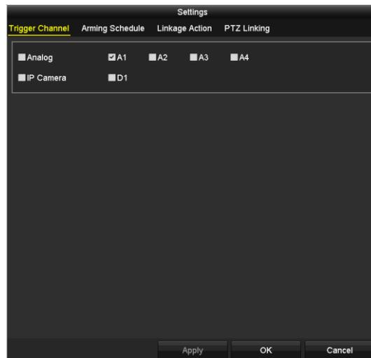
Figure 5-21 Set Triggered Camera of VCA Alarm
