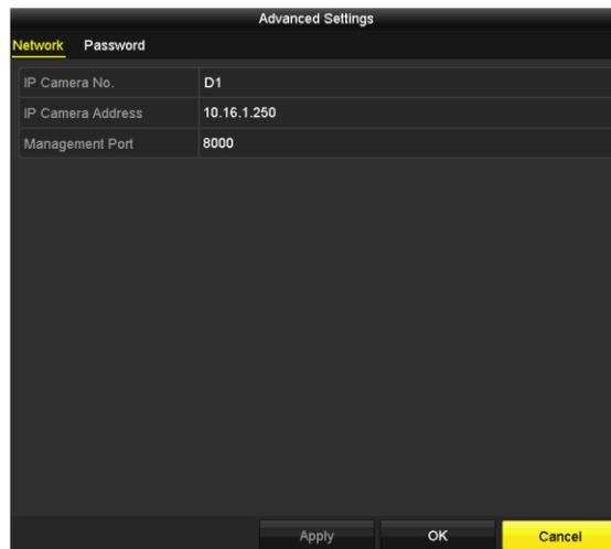
Figure 2-42 Network Configuration of the Camera
